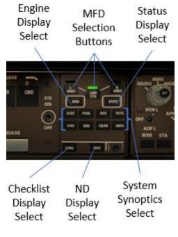
**Checklist Display Select**: Pressing this button will cause the checklist page to appear on the currently selected MFD. To simplify checklist interaction, you can click directly on the screen to interact with the checklist.
