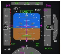
You should be prepared to disconnect the auto throttle during flare, which you can do either with the A/T ARM switches on the Glareshield MCP, or with the side button on the throttles.
