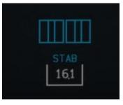
The stab pumps should be turned off if the stab tank is empty.
