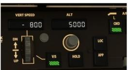
Now the plane will begin a left turn to intercept the final approach. Begin a descent to 3,000' by setting the altitude in the MCP altitude window to 3000 and once again selecting VS mode with a -800 descent rate.
