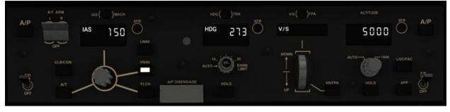
VNAV will command a climb to 5000' and TOGA lateral mode will keep you level until you engage heading mode.
