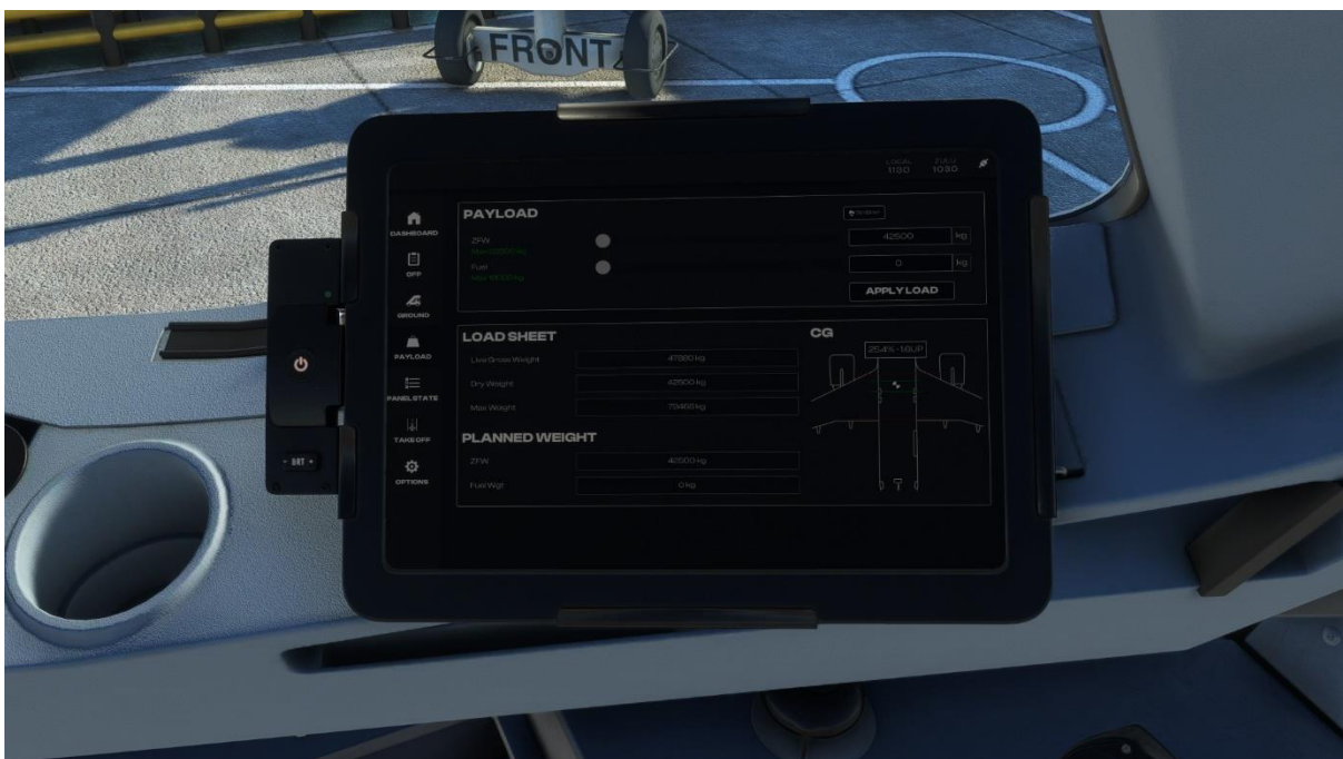
Payload Page – This page allows you to set the fuel and load on the aircraft and apply it to the FMS.
