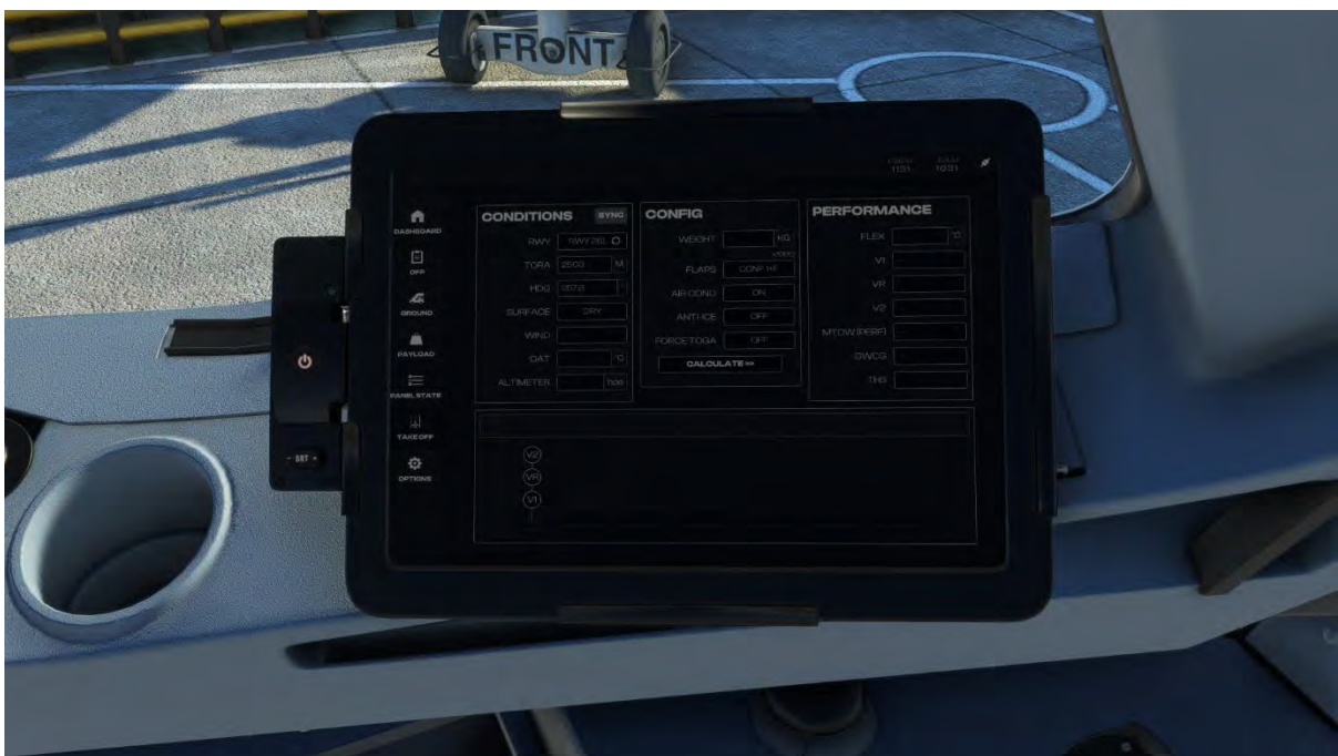
Take Off Page – This page allows you to set the conditions for Take Off to calculate your performance references.
