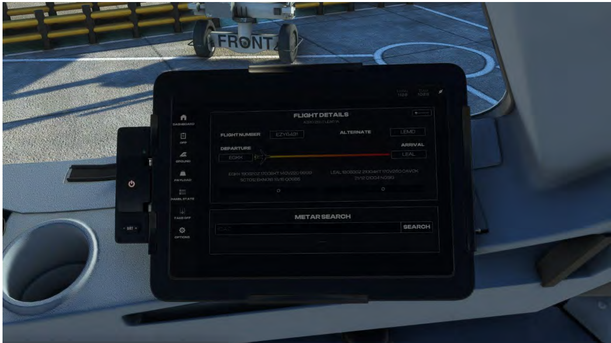
Dashboard Page – Shows your current flight details as set in the FMS, along with METAR for your departure and arrival airports. There is also a METAR search functionality.
