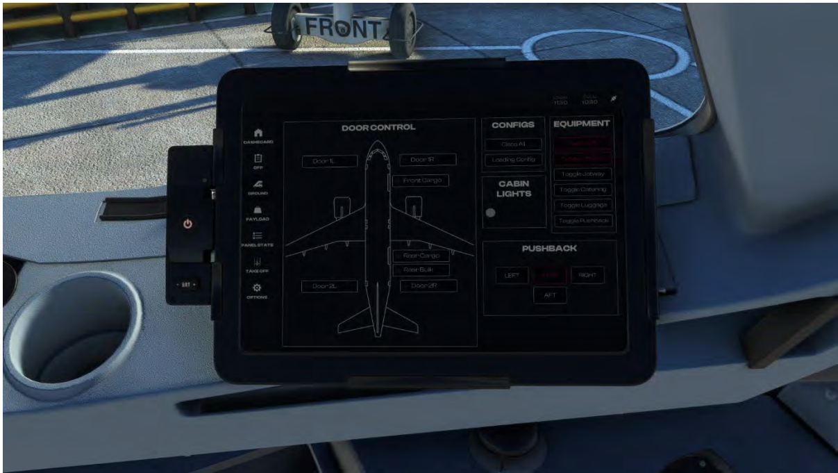
Ground Page – Controls doors on the aircraft along with requesting external Ground Services Equipment, Jetway, Pushback and manual steering of the aircraft during pushback.
