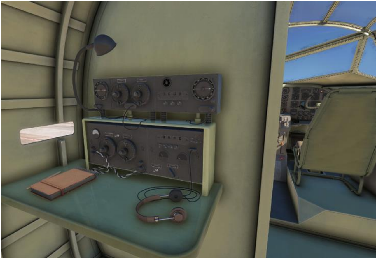
The Radio Operator console is located in the rear of the flight deck.
