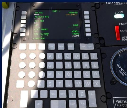
Input two ICAOs separated by / ( Bottom left of screen )
