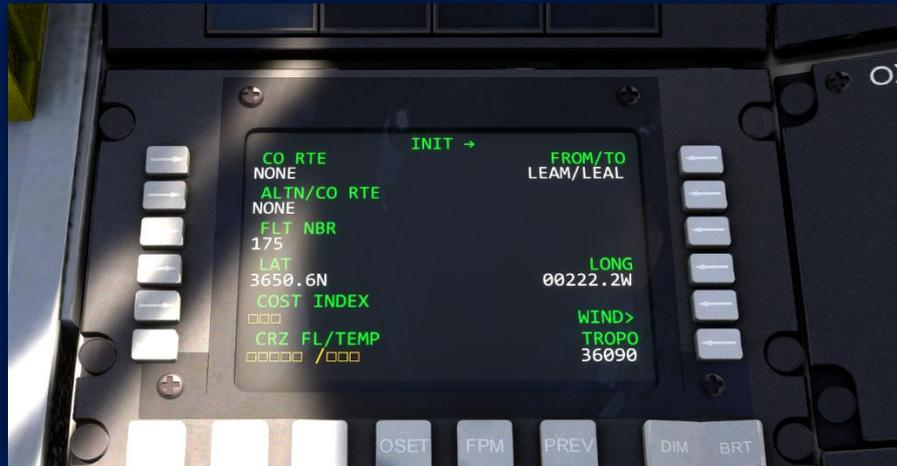
The pilot can define departure procedure, arrival waypoints, and approach waypoints. For example: pressing L1 (where FROM LEAM is) will then display details of the airport;
