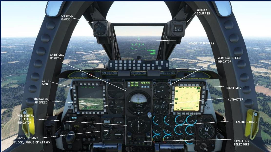
Primary flight instruments shown above. The two multi-function displays indicate pertinent navigation data, while the head-up display shows flight data through the pilot's viewing perspective. The artificial horizon and horizontal display indicator in the center of the panel provide attitude and navigational data. Airspeed, altitude, and vertical speed gauges surround the horizontal display indicator.
