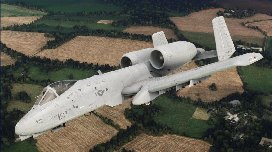
The *A-10C Thunderbolt II* is an aircraft that is relatively easy to fly. Broad, straight wings and large control surfaces give excellent response rates, and the slower flying airspeed gives the pilot more time to “get ahead of the aircraft” when compared to other modern fighter jets.
