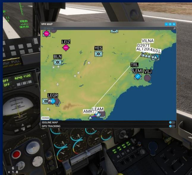
The Microsoft Flight Simulator A-10C Thunderbolt doesn't have NAV (as per the real aircraft), so the autopilot will only allow manual headings, but the HSI will mark the route for you with course and distance;
