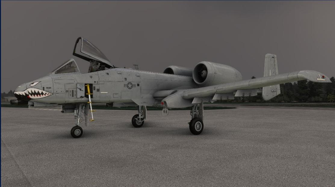
The A-10C Thunderbolt II is one of military aviation's most distinctive aircraft. Built around a rotary cannon the size of a small car, its twin turbofan engines are mounted high on its rear fuselage to mitigate foreign object debris (FOD) ingestion and its tail comprises twin vertical stabilizers.
