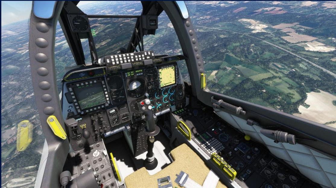
The *A-10C Thunderbolt II* has a very modern cockpit layout, familiar to most. The following pages will show the main instrument panels and features of the aircraft, as well as how to use the simulator's Interactive Checklist in order to find your way around the cockpit.
