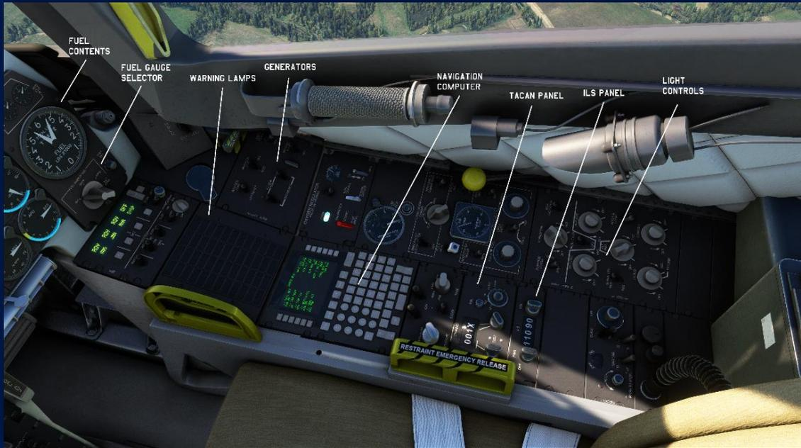
Fuel contents, fuel display selector, warning annunciators and generator switches can be found on the right-side panel. The FMC-style navigation computer can be used to input complex flight plans.
