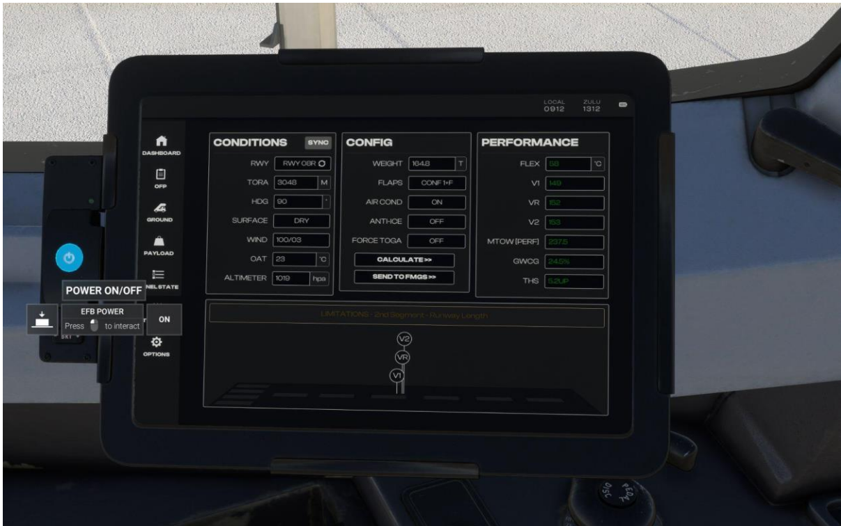
The EFB can be turned off by pressing the power button to the left-hand side of the EFB. There are also brightness buttons here to increase or decrease the screen brightness.
