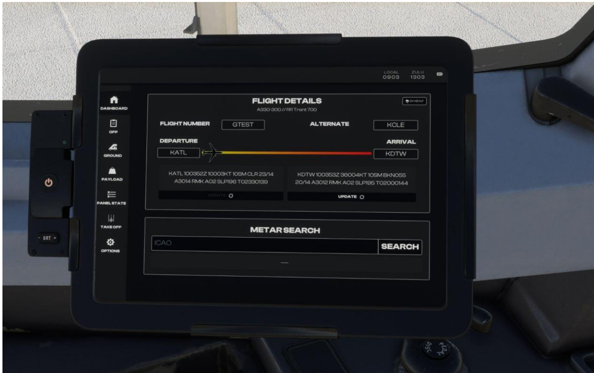
Dashboard Page – Shows your current flight details as set in the FMS, along with METAR for your departure and arrival airports. There is also a METAR search functionality.
