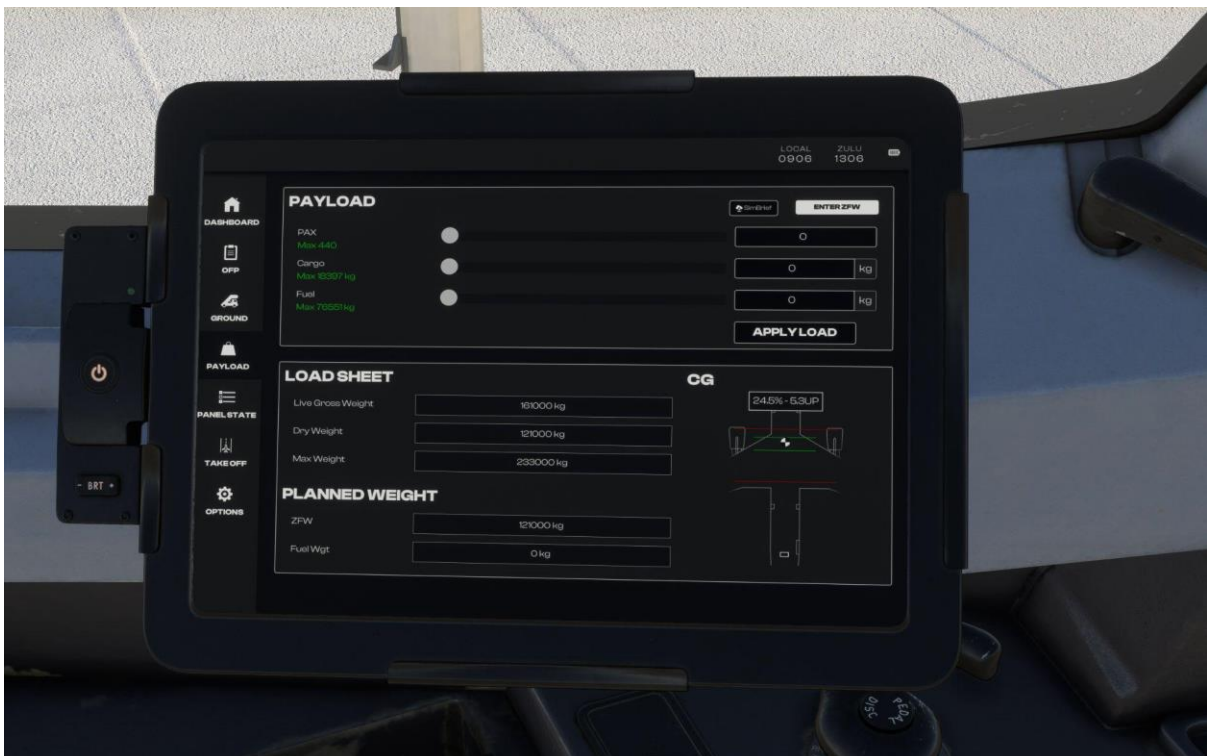
Payload Page – This page allows you to set the fuel and load on the aircraft and apply it to the FMS.
