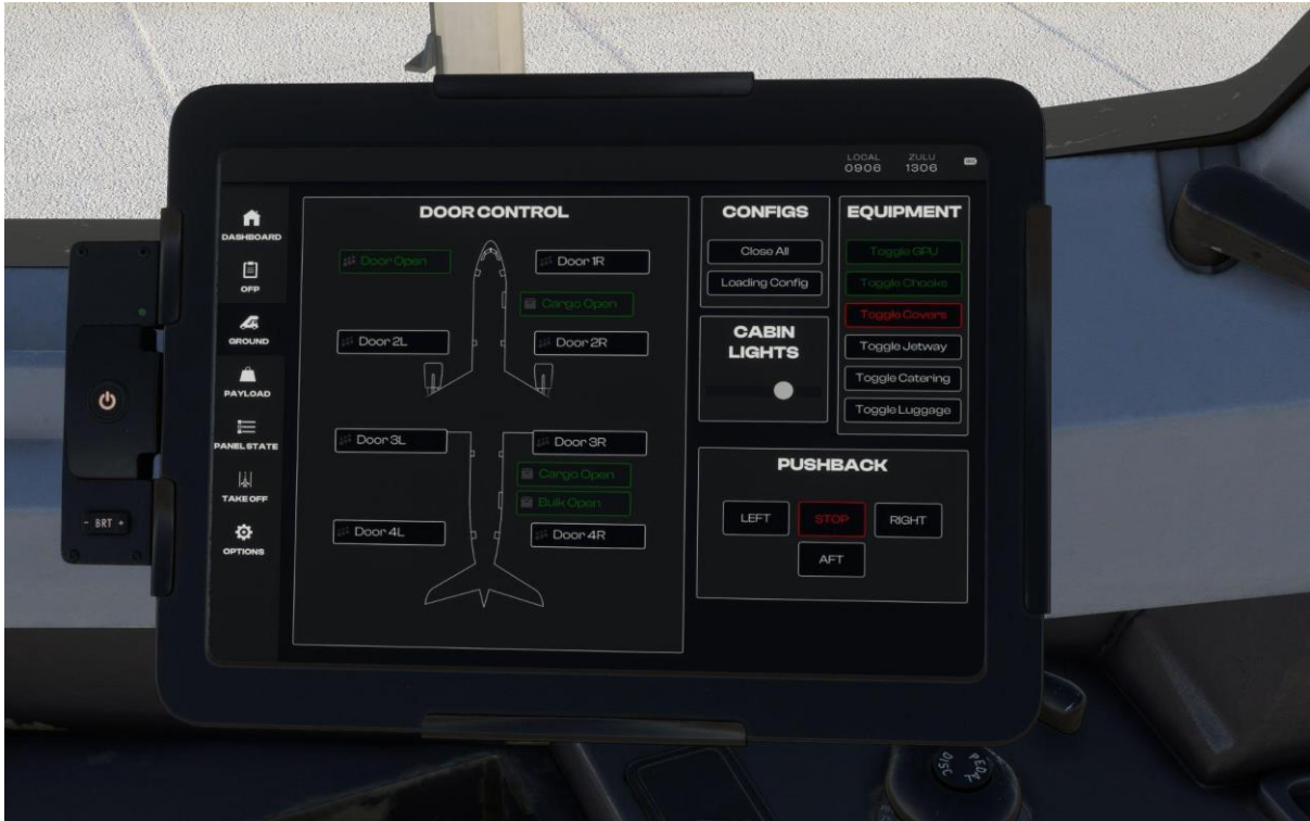
Ground Page – Controls doors on the aircraft along with requesting external Ground Services Equipment, Jetway, Pushback and manual steering of the aircraft during pushback.
