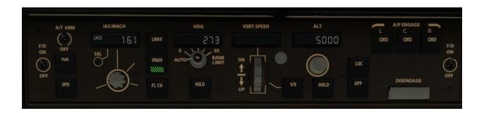
VNAV will command a climb to 5000' and TOGA lateral mode will keep you level until you engage heading mode.
