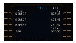
After entering an airway, you can either enter the exit waypoint in the right (TO) column, or you can enter another airway below that connects with the prior airway. In your case, since our flight plan calls for changing from airway J60 to J162 at DJB, we can simply enter airway J162 on the next line and the FMS will automatically determine that we want to change airways where the two intersect at DJB.
