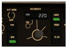
Upon reaching SIYOB descend to 5000' and reduce speed to 220 kts. To do this, first press the speed knob to display/open the speed window, then use the knob to reduce speed to 220. Opening the speed window allows you to take manual control of the target airspeed. The PFD will reflect the newly set speed in magenta.
