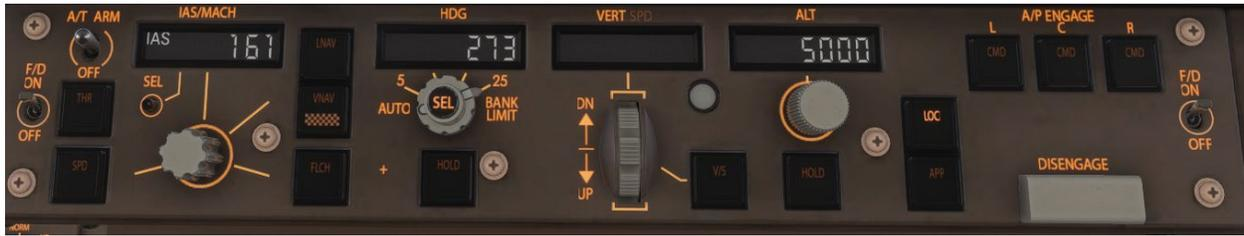
VNAV will command a climb to 5000' and TOGA lateral mode will keep you level until you engage heading mode.
