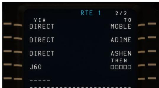
After entering an airway, you can either enter the exit waypoint in the right (TO) column, or you can enter another airway below that connects with the prior airway. In your case, since our flight plan calls for changing from airway J60 to J162 at DJB, we can simply enter airway J162 on the next line and the FMS will automatically determine that we want to change airways where the two intersect at DJB.
