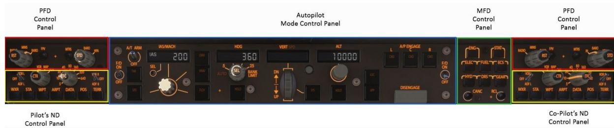
The glareshield comprises two central/shared control panels and two side-specific control panels on each side.
