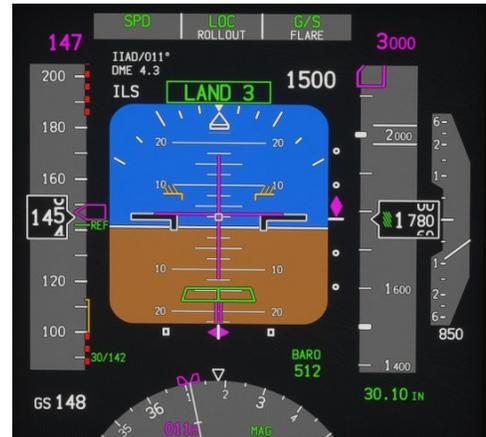
You should be prepared to disconnect the auto throttle during flare, which you can do either with the A/T ARM switches on the Glareshield MCP, or with the side button on the throttles. If using the side button on the throttles, first highlight the throttles and then right click to view the button clicking options for the throttles. If using the side button on the throttles, first highlight the throttles and then right click to view the button clicking options for the throttles with tooltips on.
