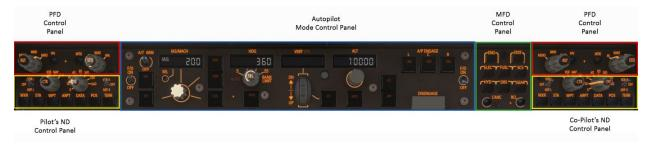
The glareshield comprises two central/shared control panels and two side-specific control panels on each side.
