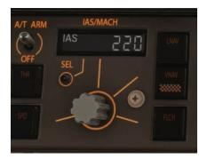
Upon reaching SIYOB descend to 5000' and reduce speed to 220 kts. To do this, first press the speed knob to display/open the speed window, then use the knob to reduce speed to 220. Opening the speed window allows you to take manual control of the target airspeed. The PFD will reflect the newly set speed in magenta.
