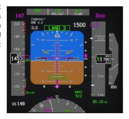
You should be prepared to disconnect the auto throttle during flare, which you can do either with the A/T ARM switches on the Glareshield MCP, or with the side button on the throttles. If using the side button on the throttles, first highlight the throttles and then left click to view the button clicking options for the throttles with tooltips on.
