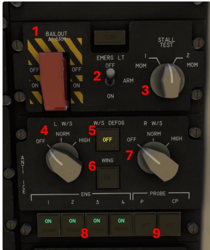
Deicing, Anti-Icing and Misc Panel
