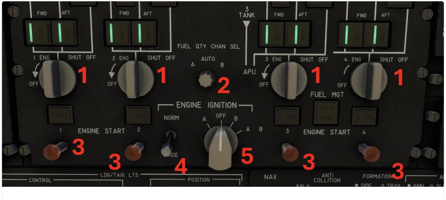
Engine Control Panel, Overhead
