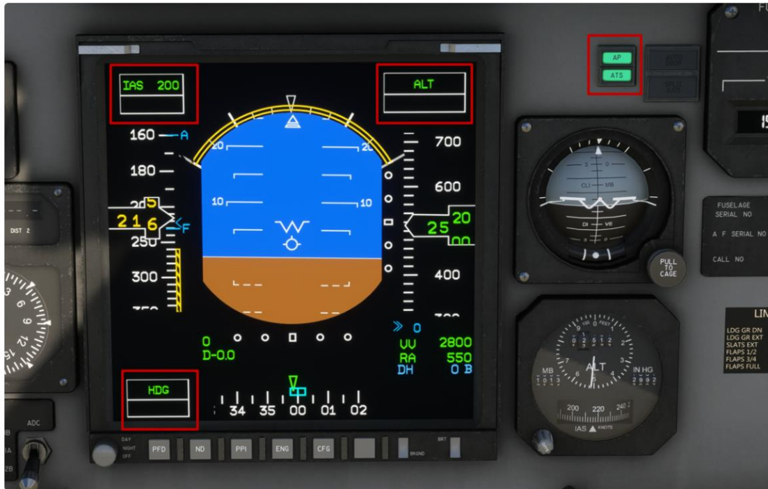
Primary Flight Display showing active modes - IAS, ALT, HDG. Notice AP and ATS lights are active, indicating the system is engaged.
