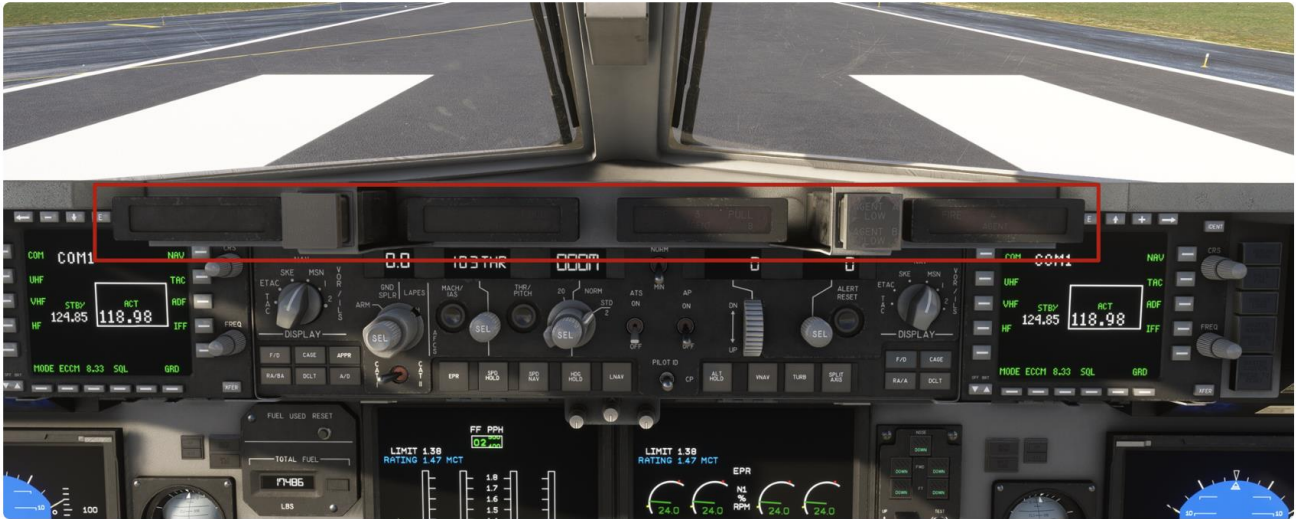
Fire Extinguisher Handles
