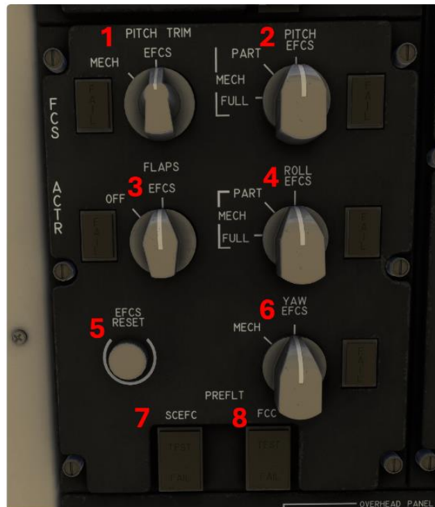
Electronic Flight Control System Panel
