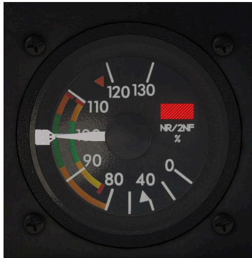
Triple RPM indicator (NR, N2 for each engine) with red failure flag
