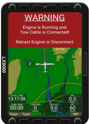
Tow Cable Unsafe Warning
