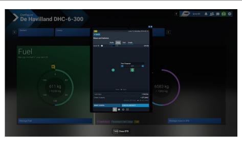
The last step to adjust the payload is to setup fuel – we intend to take 709 kg (1.563 lbs) of fuel with us, so adjust the slider or values in both center tanks accordingly. Make sure that the indicated unit is 'lbs' and not 'gal' (gallons) and that the 'Load in aircraft' button is clicked when adjustment is completed.
