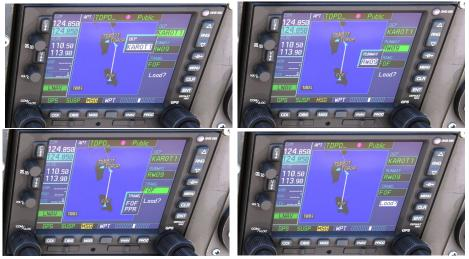
4. In case we need to add the approach as well, press the PROC button again, navigate to 'Select Approach' and press the ENT button.
