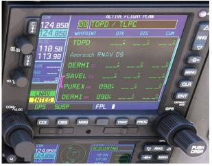
2. As the KAROT1 departure is missing, press the PROC button to open the procedures menu and navigate to line 'Select Departure' and press ENT button
