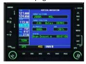
Continue the cruise and when approaching the top of descend prepare to descend. Select an altitude of 2,000 ft and change the autopilot mode to V/S (vertical speed) by pressing the ALT button to deselect altitude hold mode. When passing TOD, move the throttle levers to flight idle and leave the prop levers at the cruise setting. Adjust VS to -700fpm or according to the value displayed in the GPS VNAV mode.
