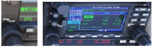
Check that 10,000ft is already selected as the cruise altitude and that the autopilot automatically levels off during climb. As the last step check that the radios are tuned to the correct stations as shown in the picture below:
