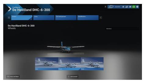
Now switch to fuel and payload and open the EFB by clicking the 'Manage mass in EFB' button in the lower right corner. We intend to transport 12 passengers, weighing 1,177 kg (2,595 lbs). Use the 'quick fill' slider to get the next value to 1,177 kg (2,595 lbs), then click on the single rows to adjust loading in detail until the total reads 1.177 kg (2.595 lbs). Then press 'Load in aircraft'.
