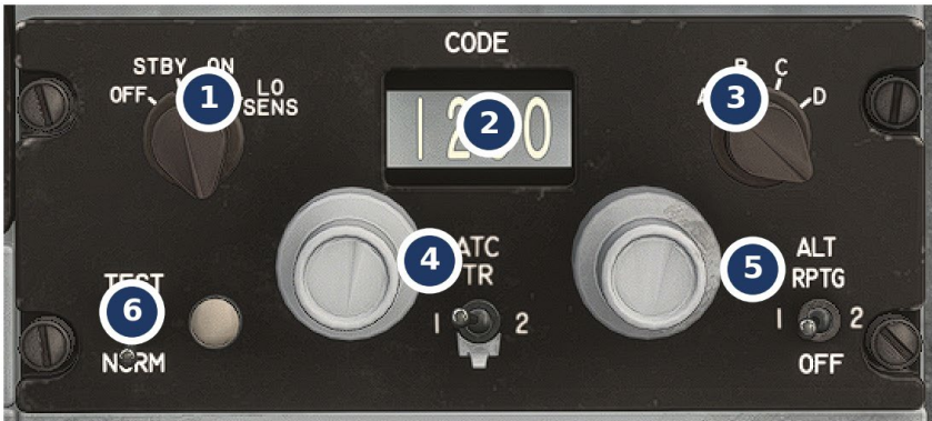
Figure 19-5 ATC transponder — mode knob (1), CODE window (2), reply-code selector (3), ATC TR selector (4), ALT RPTG (5), TEST/NORM & IDENT (6)
