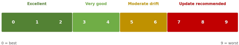
Accuracy Index (5th digit of the DSRTK/STS status word, in NAV)
