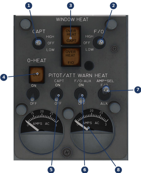
Figure 9-2 Window Heat panel — CAPT window-heat switch (1), F/O window-heat switch (2), OVER HEAT lights (3), Q-INLET HEAT switch & OFF light (4), PITOT/ATT WARN HEAT CAPT (5) and F/O-AUX (6) switches, AMP-SEL (7), AMPS AC gauges (8)
