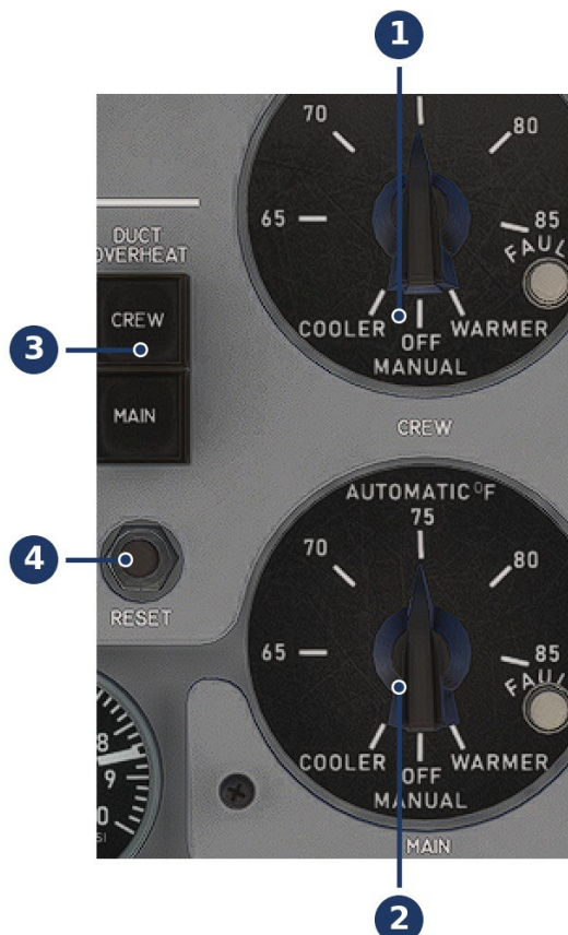
Figure 8-2 Cabin temperature control — CREW control (1), MAIN control (2), DUCT OVERHEAT test (3), RESET (4)
