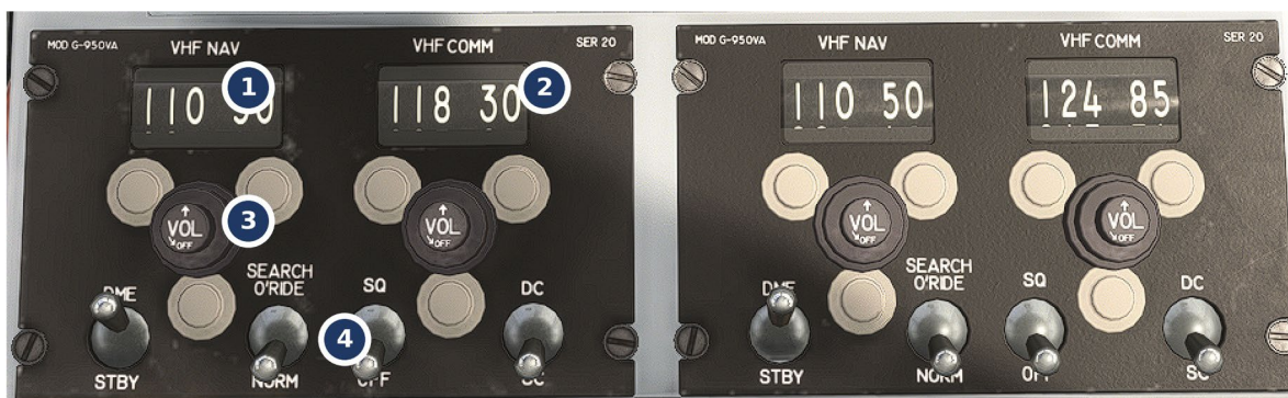
Figure 19-1 VHF NAV/COMM radios (No. 1 left, No. 2 right) — VHF NAV window (1), VHF COMM window (2), tuning/volume knob (3), function switches (4)
