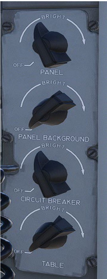
Figure 20-6 Flight Engineer Station — Lighting Controls
