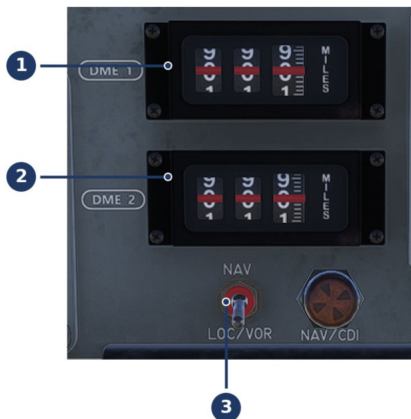
Figure 16-3 DME indicators and the HSI NAV/CDI switch — DME 1 (1), DME 2 (2), NAV – LOC/VOR switch (3)
