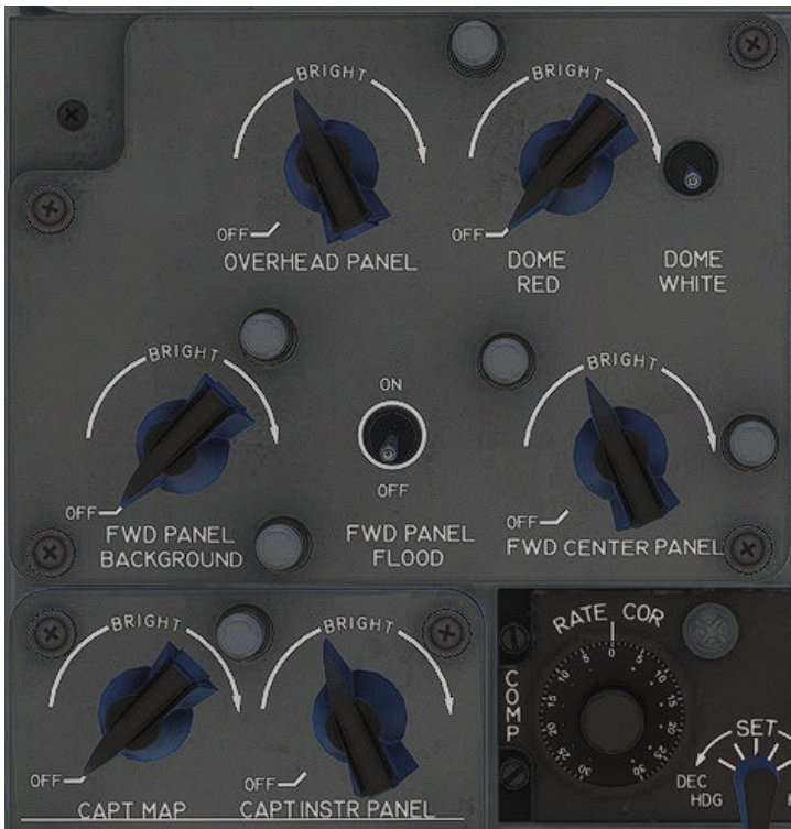
Figure 20-2 Overhead Panel — Captain's Side Lighting Controls
