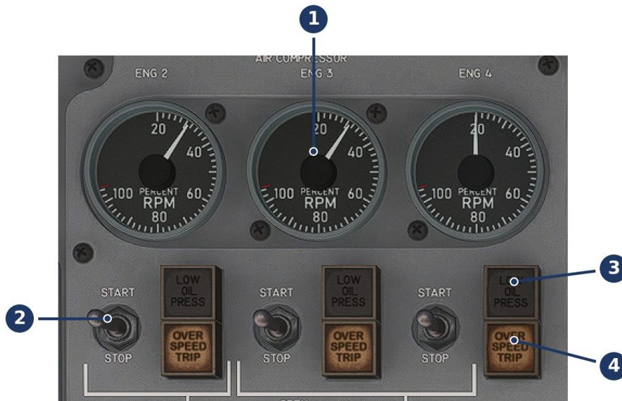
Figure 7-2 Turbocompressor controls — RPM gauge (1), START/STOP (2), LOW OIL PRESS (3), OVER SPEED TRIP (4)
