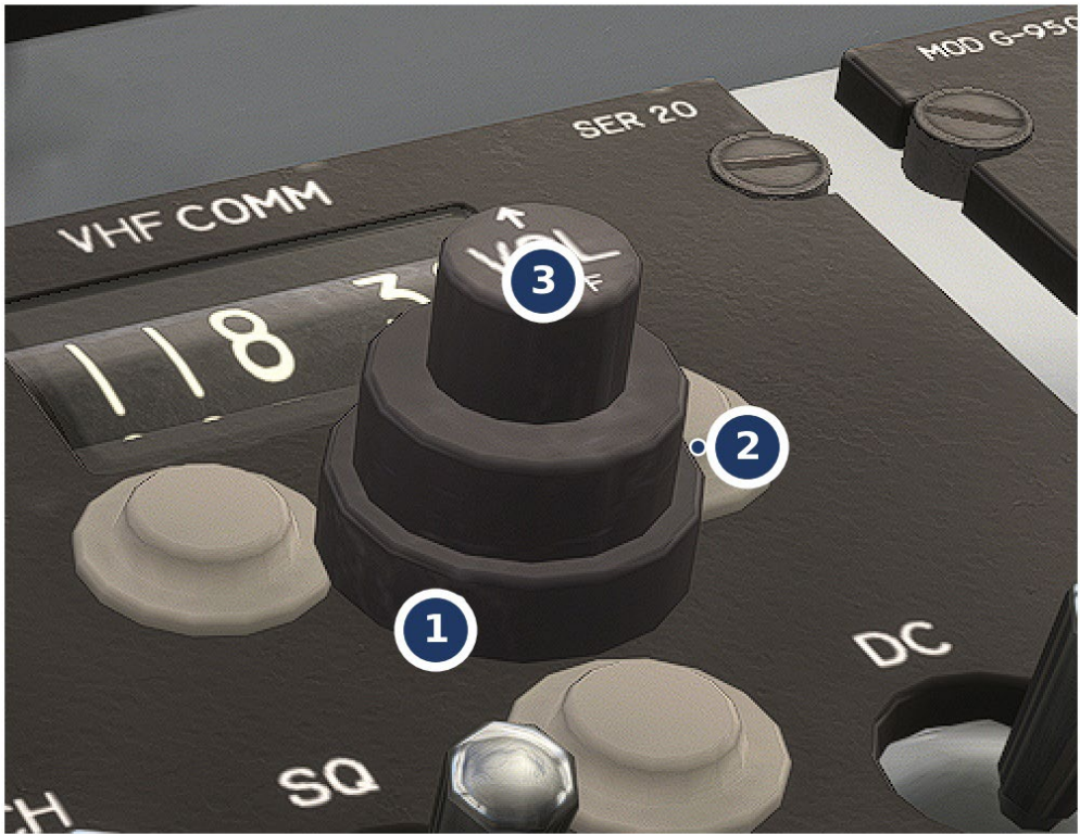
Figure 19-2 Concentric tuning/volume knob — outer/MHz ring (1), middle/decimal ring (2), inner VOL knob (3)
