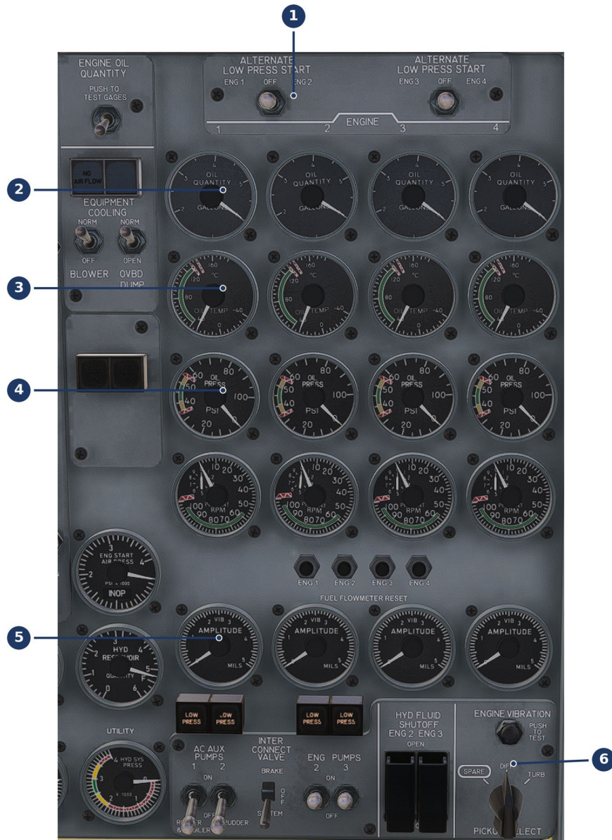
Figure 5-3 Flight Engineer's engine panel (engine-1 instruments called out; repeat for engines 2–4)
