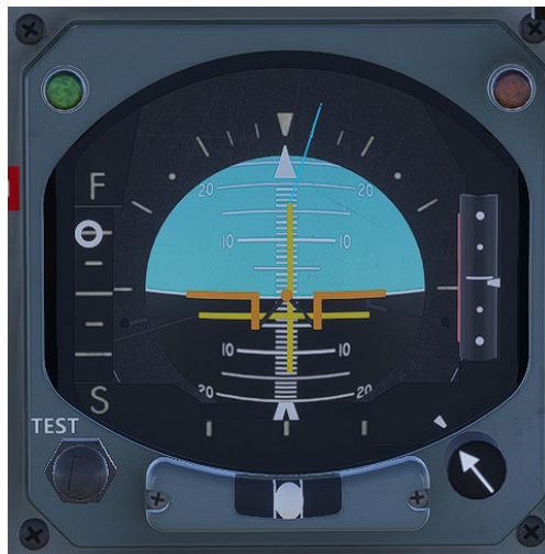
Figure 26-10 Captain's ADI — Takeoff/Climb Throttle Assistance Indicator
