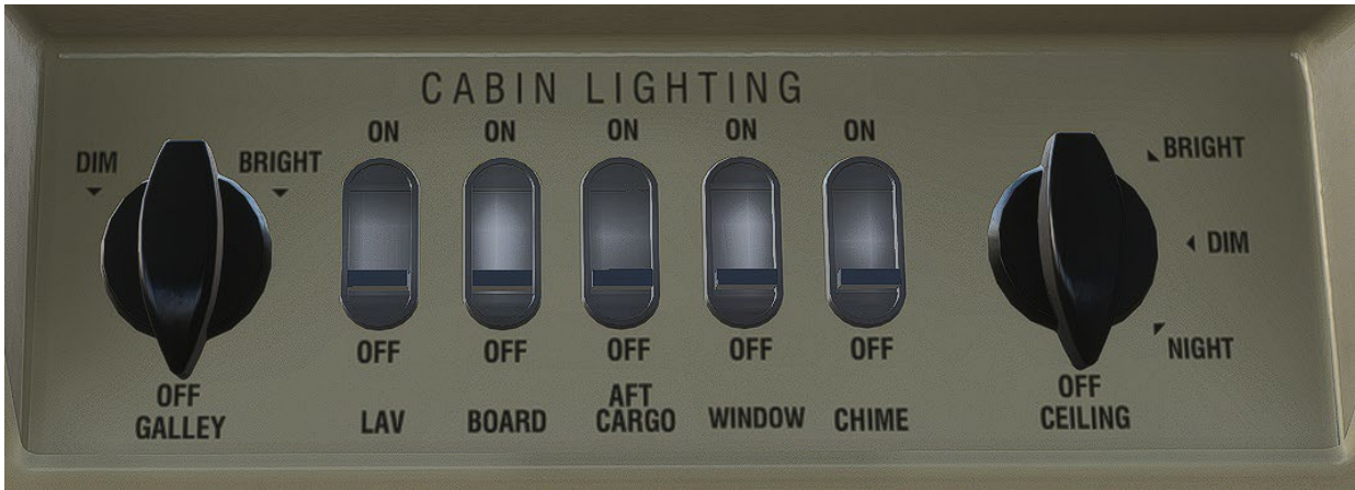
Figure 20-9 Cabin Lighting Panel — Aft Galley
