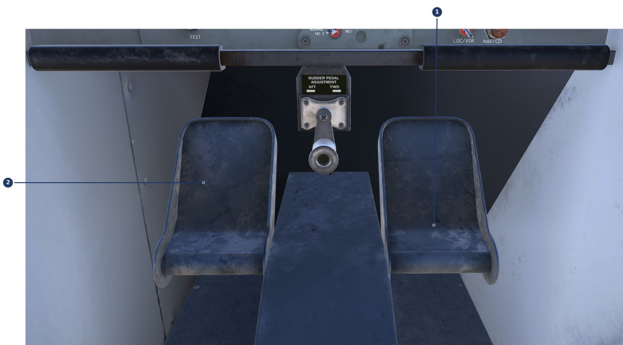
Figure 14-2 Rudder pedals — pedals translate for rudder control (1); pivot at the top for differential braking (2)
