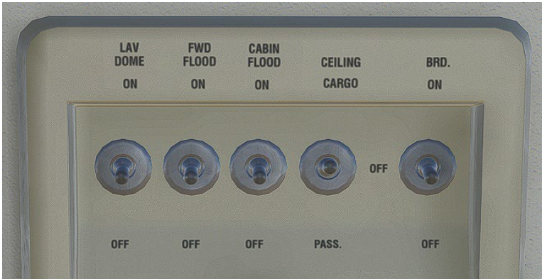
Figure 20-7 Main Cargo Lighting Panel — Forward Cabin Entry
