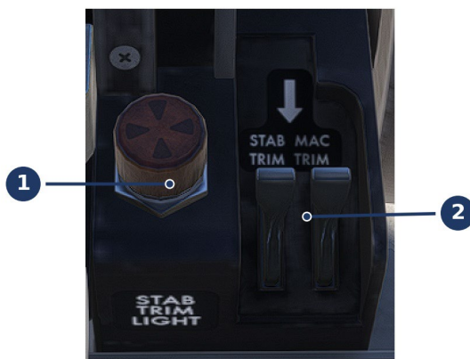
Figure 14-6 Trim-in-motion light (1) and electric-trim cutout switches (2)
