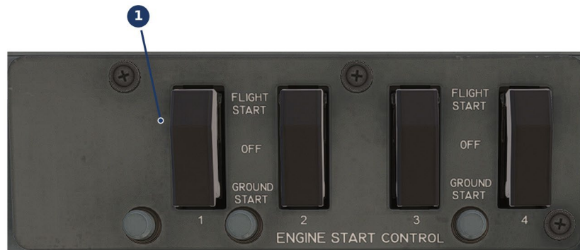
Figure 5-4 Engine Start Control panel — per-engine start switch (1); FLIGHT START / OFF / GROUND START
