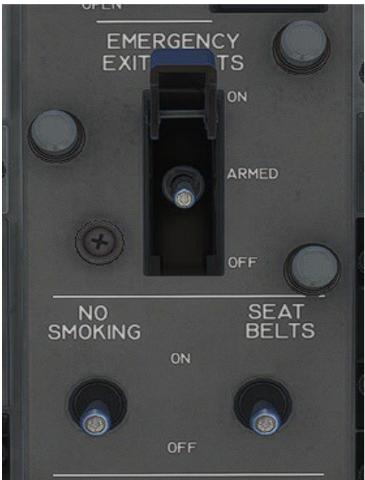
Figure 20-10 Overhead Panel — Emergency Exit Lights, No Smoking, Seat Belts
