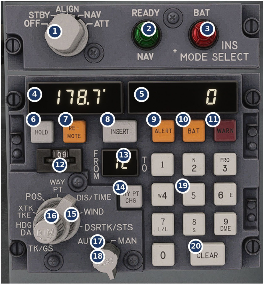
Figure 23-1 Carousel IV-A CDU / MSU — controls and indicators
