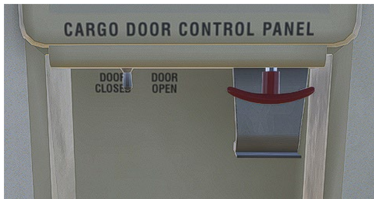
Figure 3-3 Cargo door control panel
