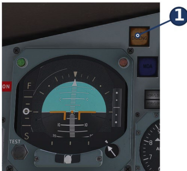
Figure 16-9 ADI with the AP DISENG warning light — AP DISENG light (1)
