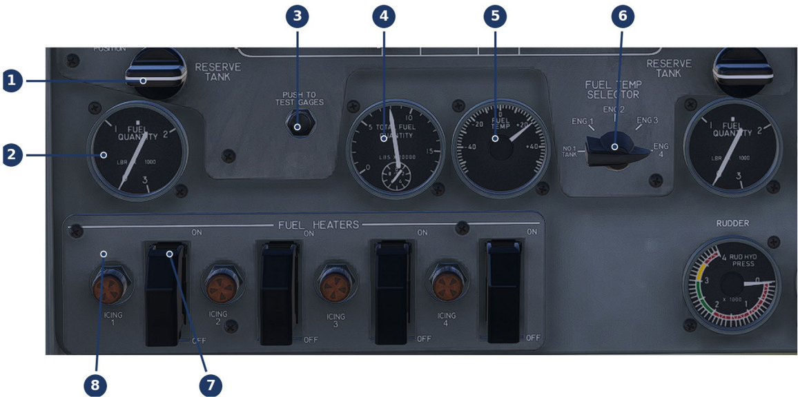
Figure 11-3 Reserve, gauge-test, fuel-temperature and fuel-heater controls
