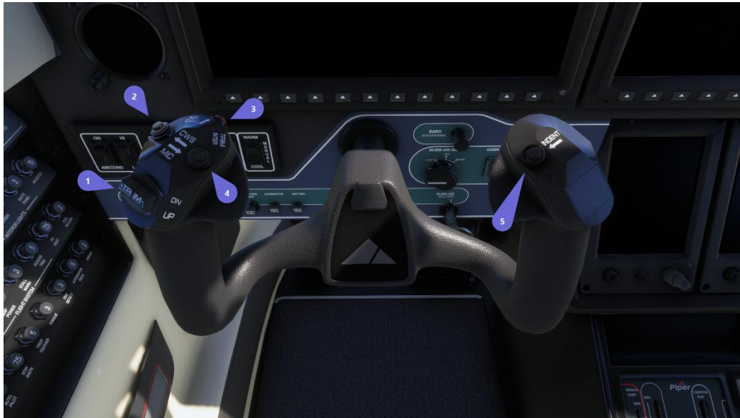
FIGURE 4-8: CONTROL WHEEL (YOKE)
