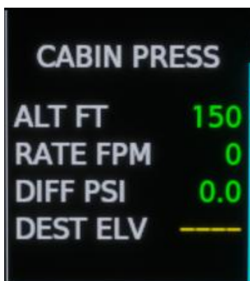
FIGURE 5-10: PRESSURISATION SYSTEM INSTRUMENTS
