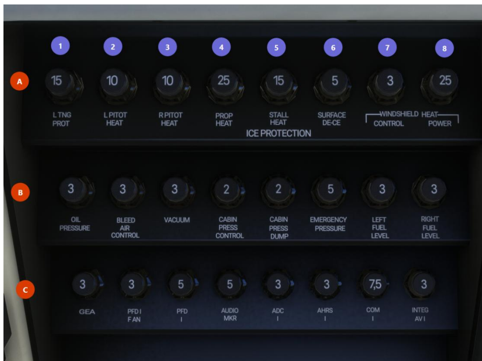
FIGURE 5-6: PILOT SIDE, AFT CBs (MAIN BUS)
