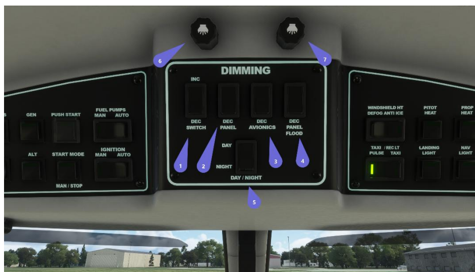
FIGURE 4-5: OVERHEAD DIMMING SWITCHES
