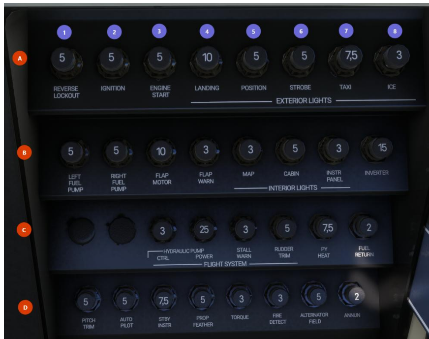
FIGURE 5-7: PILOT SIDE FORWARD CBs (MAIN BUS)
